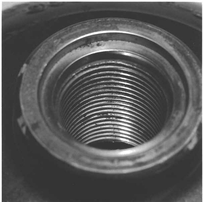
PHOTO 8. A crack in dirty threads. Threads need to be cleaned before the visual inspection begins. (See NOTE 9.)
