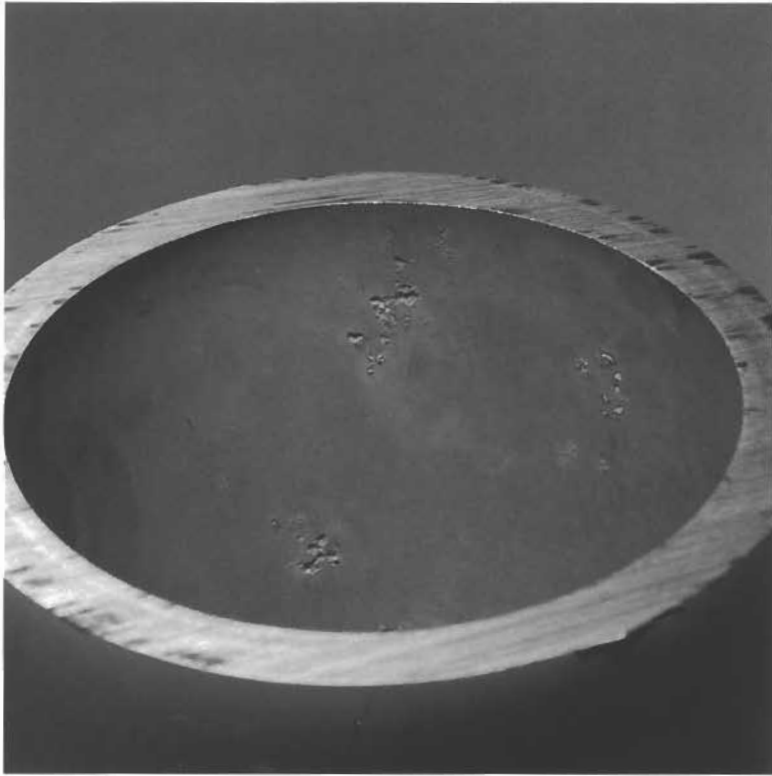
PHOTO 11. Pit corrosion in the cylinder sidewall, distant view.
