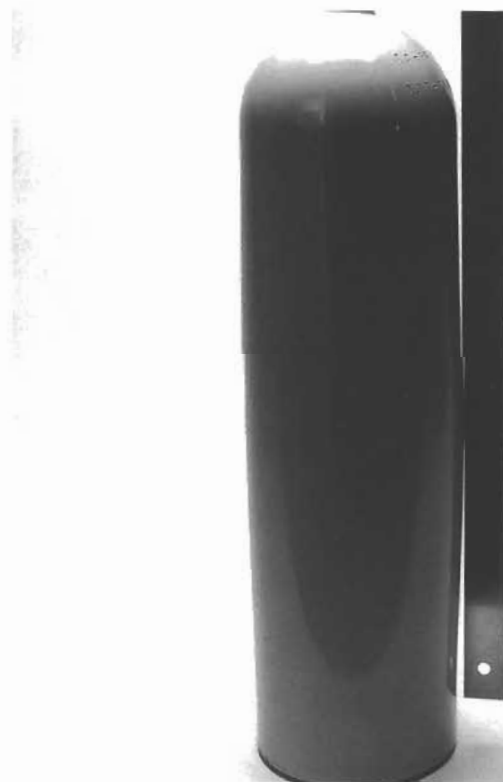
PHOTO 18. Cylinder with bow or "banana." The bow shows easily with a straight edge placed along the length of the cylinder (see FIGURE 11 of a bow 'from the other side').
